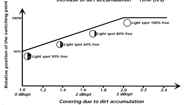
By way of continuous monitoring of the maximum value at the receiver a dynamic correction of the switching threshold compensates the effect of dirt accumulation. This means that increased dirt accumulation does not lead to a shift of the switching point.
